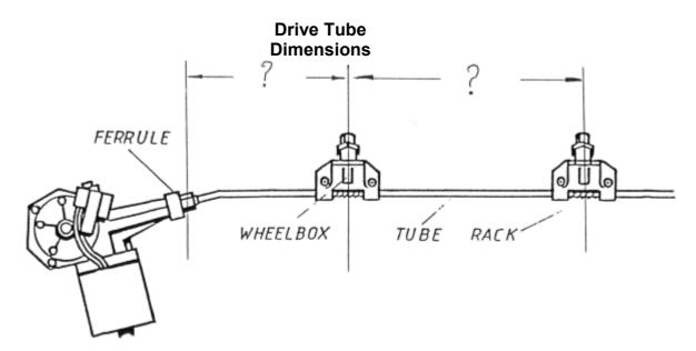
The above diagram is for self parking to be either on the left or the right sides of the winscreen. To have center parking one wheel box is fitted with bundy tubing running to the top of the wheel box. I.E. The wheel box is fitted upside down I.E turned 180 degrees. If the Wiper motor is mounted on the Passenger side then the R.H. Wheelbox is the one that needs to be fitted upside down.
